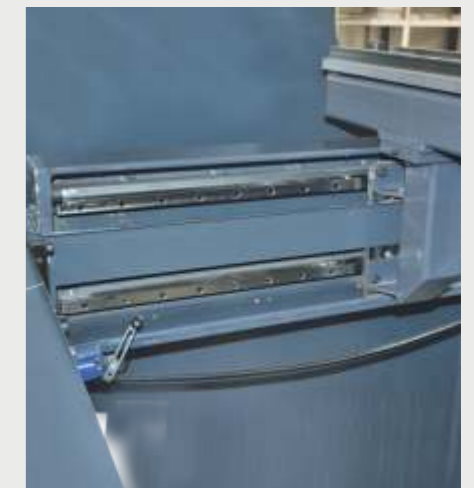
Linear Guided Stronger Back Gauge X Movement
