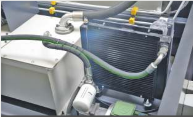
Hydraulic Oil Cooling System
