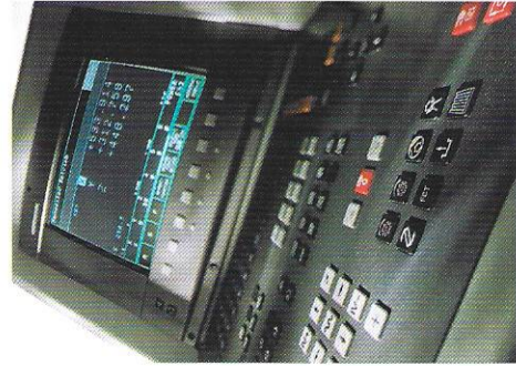
Controllo Heidenhain TNC 430.
